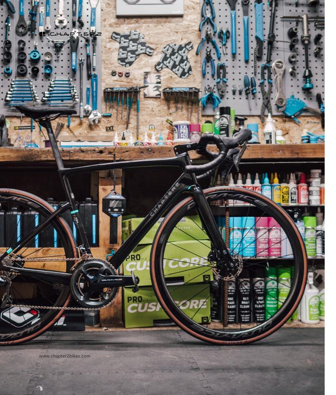
Sporting a T47 Bottom Bracket for easy maintenance, the aluminium BB Shell works in unison with the high-tensile carbon carefully laid into the BB area to increase stiffness by up to 8% over the TERE. Additionally, the use of a Latex mandrel for the whole front triangle has increased the Headtube stiffness by 34% over the TERE for that out of the saddle and power to the pedals moment.
