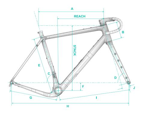
The KAHA features a Gravel Racing geometry designed for balance and stability at speed across any terrain. The double dropped chainstays delivers tire clearance up to 47mm.
